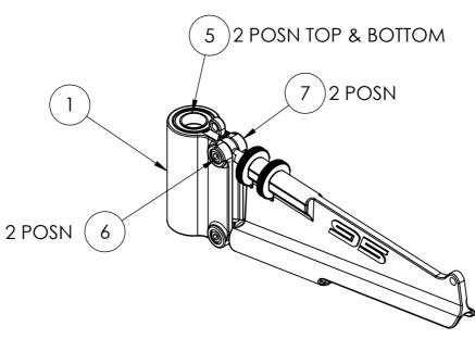
INSERT BEARING ITEM 5 IN EITHER END OF THE BEARING HOUSING ITEM 1, THEN FIT THE ASSEMBLED COMPRESSION STRUT ITEM 1, USING THE HEX SKT SCREWS AND NUTS, ITEMS 6 & 7. A 1.5mm ALLEN KEY WILL BE REQUIRED.
