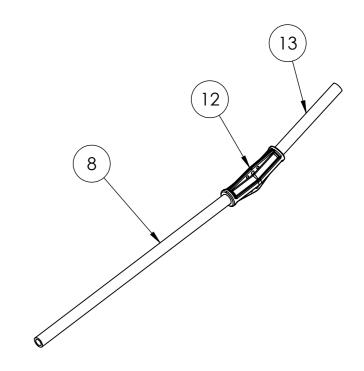
APPLY A SMALL AMOUNT OF A GLUE OF YOUR CHOICE (SUPER GLUE (CA) IS ACCEPTABLE) TO ONE END OF EACH TUBE ITEMS 8 & 13. SLIDE THE TUBE INTO THE TUBE JOINER, ITEM 12, AND HOLD TILL SET.
