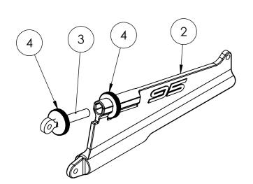
SCREW ITEM 3 EYE BOLT INTO ITEM 4 KNURLED NUT. WITH THE REMAINING KNURLED NUT, ITEM 4, POSITIONED AS SHOWN, INSERT THE ASSEMBLED ITEMS AND ROTATE THE SECOND KNURLED NUT UNTIL THE EYE BOLT ASSEMBLY IS RETAINED.
